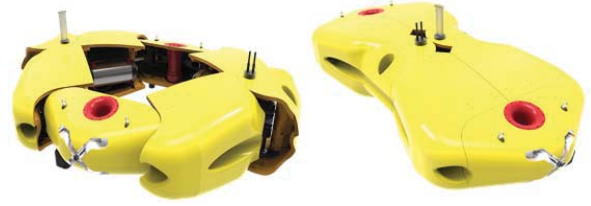
Fig. 1. The UNIFI DIF AURV in the hovering and survey configurations.
